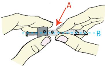
4 a. Replace the nebulizer body into the fitting, lining up the threaded holes with the indentations in the nebulizer body.
