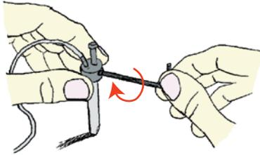
1. Holding the nebulizer in the left hand and leaning it vertically on a smooth flat surface, loosen the 2 grub screws with the right hand, using a small hex key.
