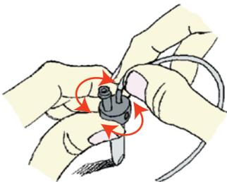
5. Holding the nebulizer in the left hand again, insert the new sample tube by twisting left to right and pushing it in gently, until it stops.
