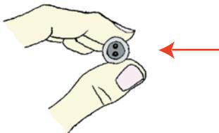
3. Check that the 2 o-rings in the nebulizer fitting are in place.
