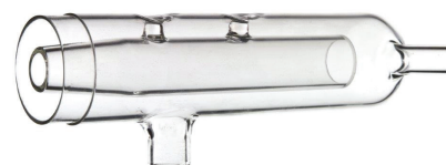
Figure 1b. Design features of the Twister cyclonic spray chamber
