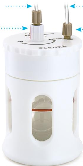
An Argon Humidifier is commonly used in ICP analyses involving samples with high concentrations of dissolved solids. It helps to alleviate salt deposits in the nebulizer and torch injector, allowing uninterrupted and maintenance-free operation.
