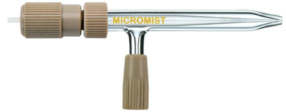
A specially designed nebulizer based on our popular MicroMist, designed to efficiently nebulize very small sample volumes at low sample and argon gas flow rates. It is a standard component of the High-Efficiency Sample Introduction System (HE-SIS), widely adopted by leading research organizations and instrument manufacturers for single-cell, single-particle, nanoparticle, and low-volume sample studies, achieving up to 95% transport efficiency when combined with the HE-SIS.
