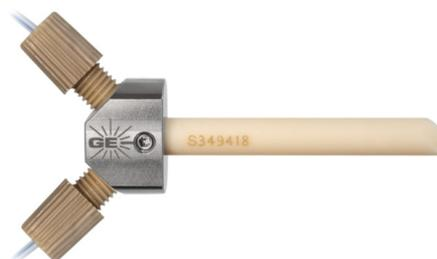
The Ceramic VeeSpray is a highly durable, V-groove design, capable of handling high levels of dissolved solids and particulates without clogging. The ceramic body is compatible with all aqueous and organic solvents, including HF. Since the VeeSpray is not a concentric nebulizer and does not self-aspirate the sample, it requires sample delivery via peristaltic pump and operates best at higher sample flow rates (1.5 – 2.5 mL/min) to reduce pulsations.
