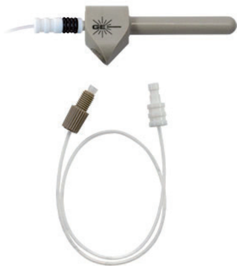
Figure 4. DuraMist DC nebulizer with PerkinElmer Avio gas fitting
