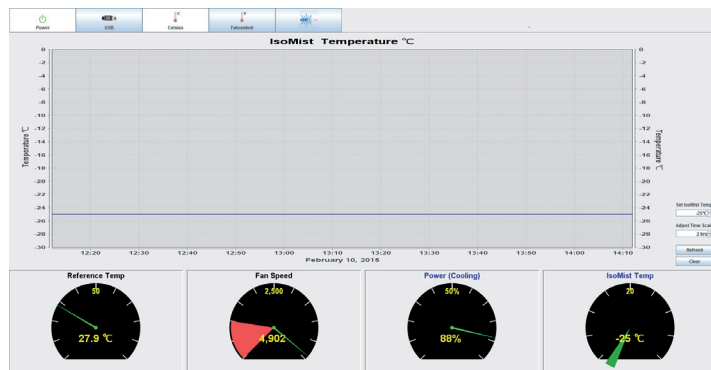
Figure 5. IsoMist™ control panel with temperature scale.
